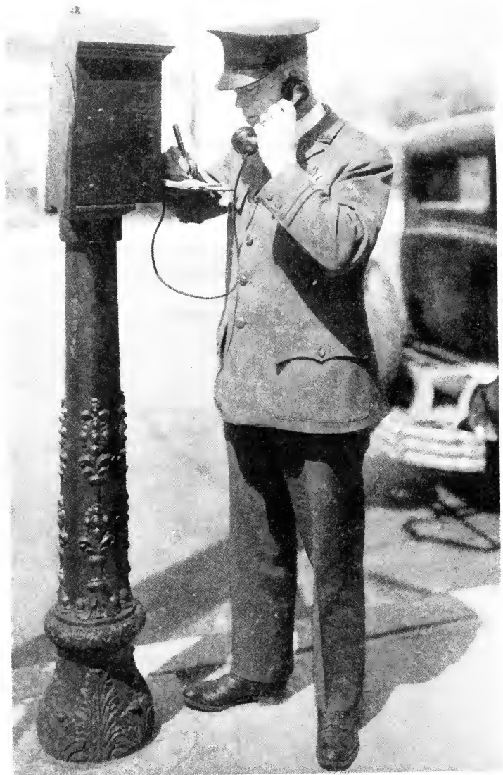
Beat telephone equipment in use. Note folding writing platform; also combined receiver and transmitter set.
